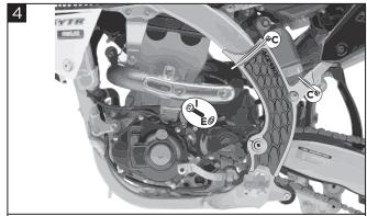
Place the X-Grip. Tighten the screw (I) and the washer (E). Fix
